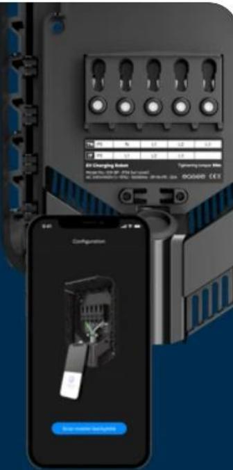
The image shows a smartphone held in front of an Easee charging backplate. The phone's camera is scanning an NFC tag attached to the backplate. The phone screen displays a 'Configuration' screen with a 'Scan NFC tag' button.
